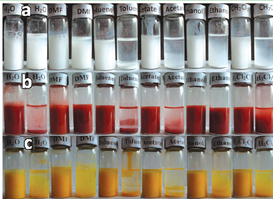
Figure 8. Photograph of dispersion of pigments in different solvents with (left) and without Z-SiPEA211 (right): (a) Titanium White; (b) Iron Red; (c) Chrome Yellow, the concentration of pigments and Z-SiPEA211 is 10 and 5 g/L, respectively. The pictures were taken after the samples were stirred for 30 min and then stood for 30 min.
